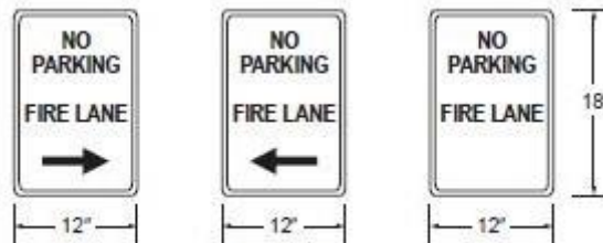
FIGURE D103.6 FIRE LANE SIGNS
